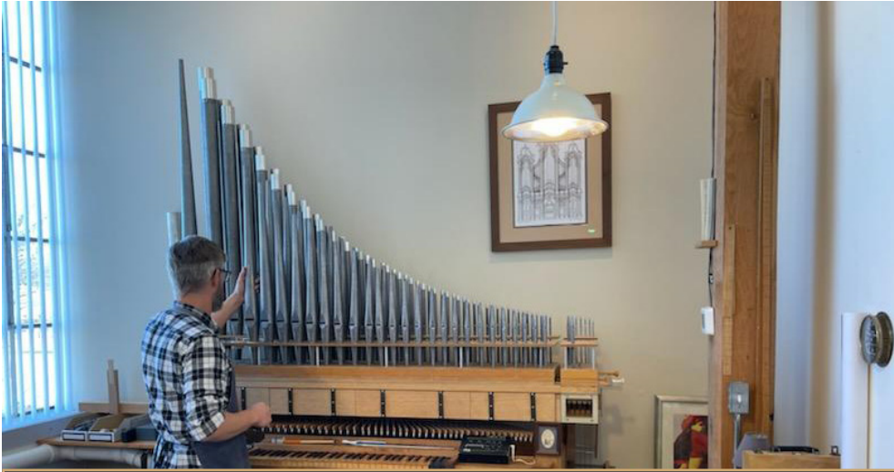
Joel VanderZee of Taylor and Boody testing the rank of the 4' Spitzflöte for tone quality. He had just finished assembling the pipes before this photo was taken.
