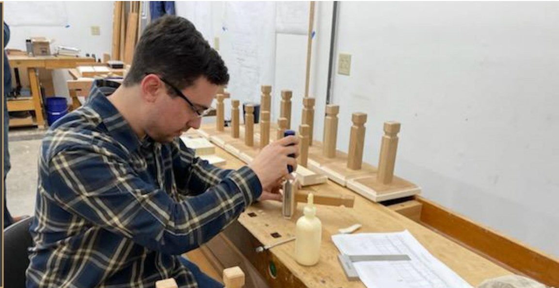
Joel VanderZee of Taylor and Boody testing the rank of the 4' Spitzflöte for tone quality. He had just finished assembling the pipes before this photo was taken.
